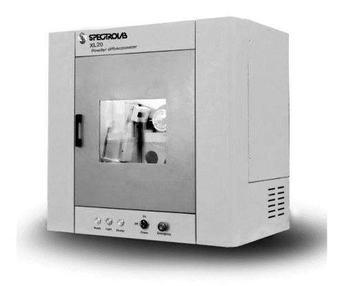
The XL-20 Desk Top Xray Diffractometer A rugged desk top XRD for routine crystalography
