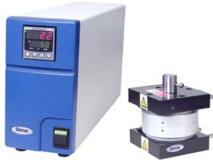
The Atlas™ Heated Platens P/N GS15515 fit into all of the Specac Atlas™ hydraulic presses as standard. This accessory converts a press to offer a heated surface of 100mm diameter for pressing at temperatures up to 300°C and a maximum load of 15 tons.
